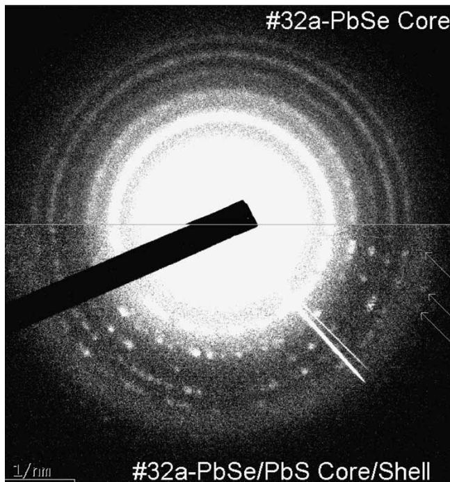
Figure 3. Selected-area-electron-diffraction (SAED) patterns of plain-core PbSe (upper half) and core-shell PbSe/PbS nanocrystals (lower half).
